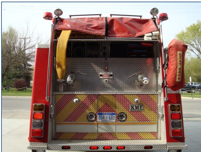
(Left) Hose bed storage compartment was modified to fit backboards and hand tools.
